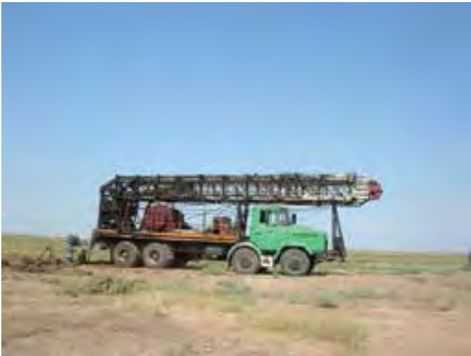
Service Rig Moving to Work Over Well with ESP
