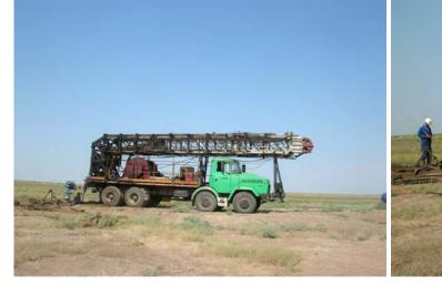
Service Rig Moving to Work Over Well with ESP
